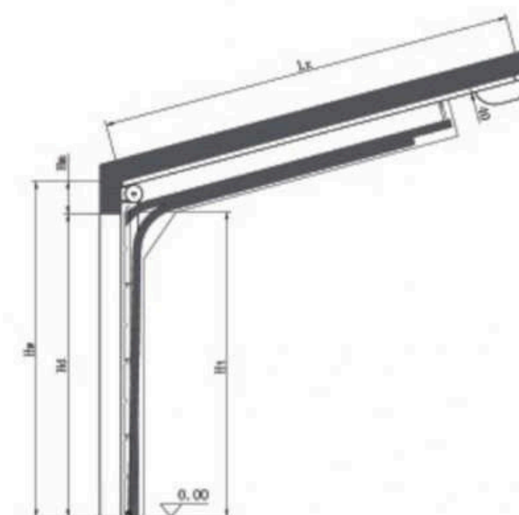
Slant horizontal tracks' installing-double tracks
