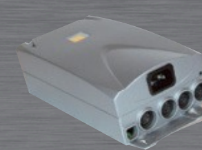
Main Programmable Controller
